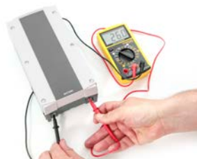
Checking voltage on battery
