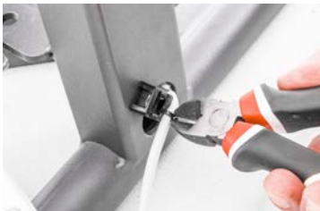
Cutting the cable tie
