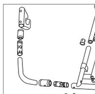
Individual brackets can be replaced by the removal of two countersunk socket head screws. Removing additional screws with break down the chair bracket arm into individual components if replacement is required.
