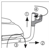
Ensure that all four brackets can rotate and lock properly as indicated. ① Bracket raises and locks ② Bracket extends and locks ③ Bracket rotates and locks ④ Bracket rotates and locks.
